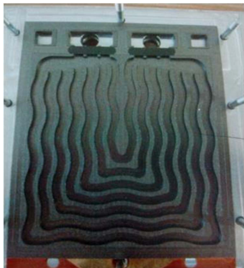
Figure 2. Construction of our improved anode for usage in laboratory scale MFCs.
