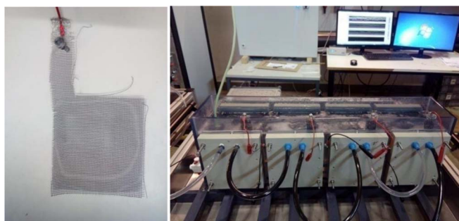
Figure 3. Stainless steel mesh with graphite plus \text{MnO}_2 composite (left) and in series connected smaller laboratory scale MFCs (right) ( 150 \text{ mm} \times 150 \text{ mm} ).
